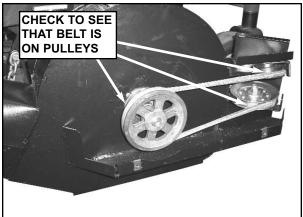
**STEP 6b:** Check to see that blower belt is routed around impeller pulley and idler pulleys after belt is installed onto deck pulley. Replace cover, tightening bolts securely. **IMPORTANT:** Never operate any mower without a pulley guard securely in place.
